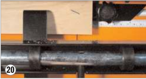
20. Add the Clamp Extension Arm and butt the stiles labeled with a 1 horizontally against the stop and cut a dovetail socket.
