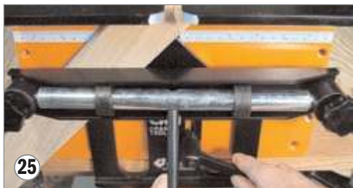
25. Slide the Miter Plate against the bottom edge of the mitered piece and lock the Miter Plate in place.
