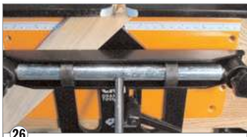
25. Slide the Miter Plate against the bottom edge of the mitered piece and lock the Miter Plate in place.
