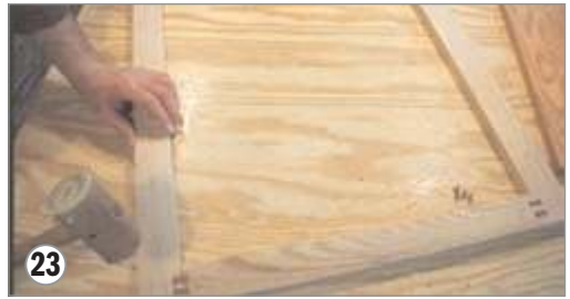
23. Assemble the frame by inserting the keys and tapping the caps in place.
