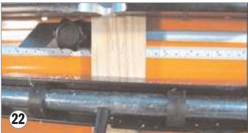
22. Reposition the stop, using the same settings as on the right side , on the left side and repeat the process, placing parts labeled with a 2 against the stop in this position.
